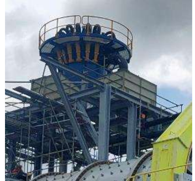
Cyclone to separate the fine ores (-75 um) from the coarse ores (+75 um)
