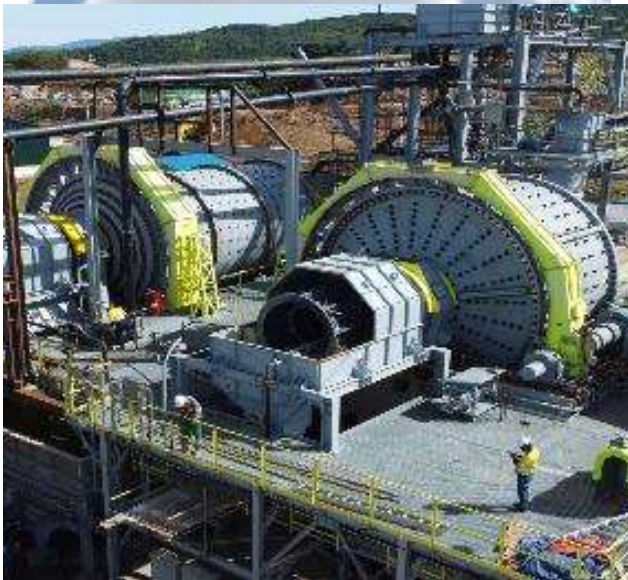
Sag mill and Ball mill grind the ores from size 12 mm to become 75 um
