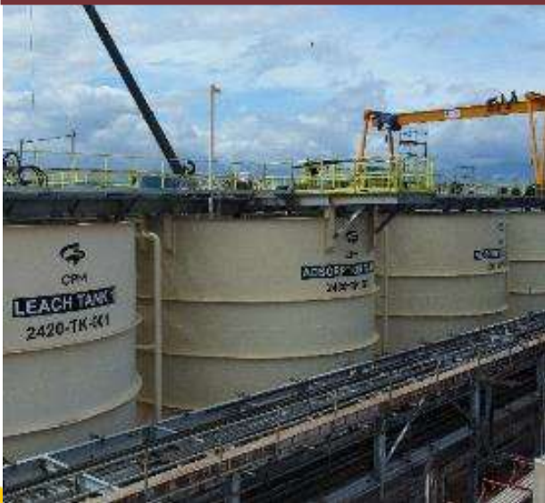
Carbon in leach tanks to extract the gold & silver contents from the ores by using cyanide
